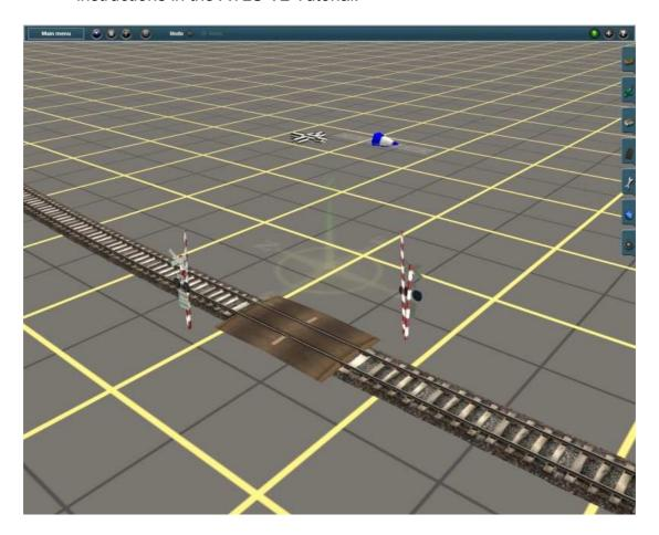
2) Using the Split Spline tool, disconnect the track from both sides of the crossing and using the Move Tool, move the track to one side.
